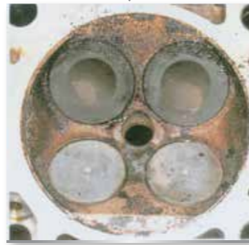
Deposits and corrosion of the valves
