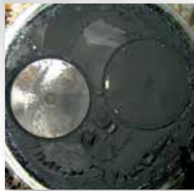
Carbon deposits on valves
